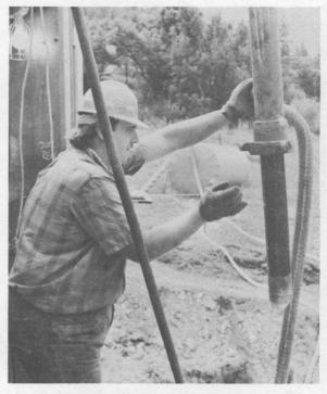
TIP OF CORE SAMPLE is visible at end of core tube. Tonto's Jeff Riley has his left hand on the loading chamber that provides blow-out prevention even when a core tube is being removed from the corehole. Jeff and other members of drill crew received special training in BOP operations.
